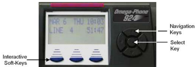
OM-KTD30 Interactive Soft Keys and Navigation Keys
